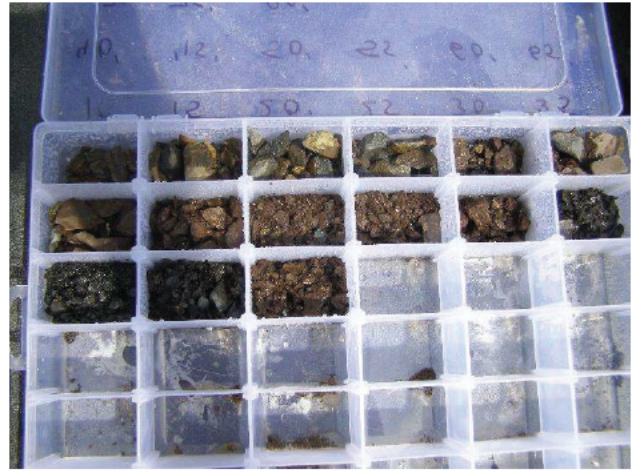
Photo 2: Rock chips collected from 5-foot intervals during drilling
