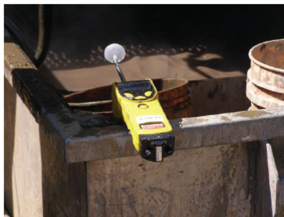
PID near drilling rig 5-4-26 @ 10:25
