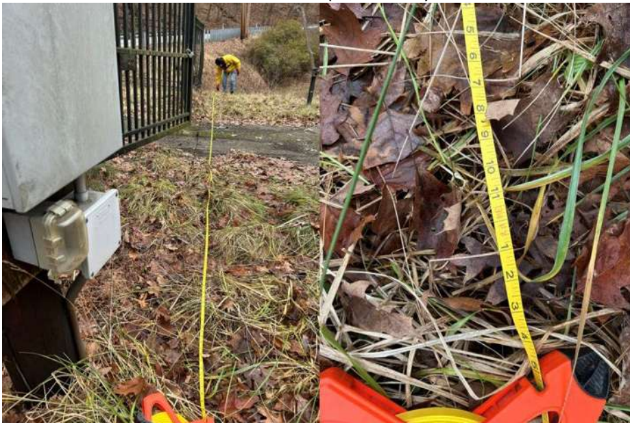
Photo 3 and 4: Measurement of clear width at gate. (1-13-2026)
