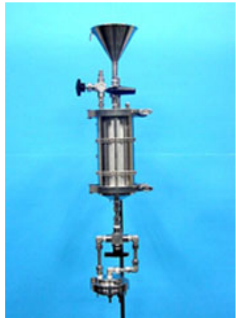
Pressure Filtration Vessel
