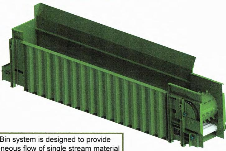
The Metering Bin system is designed to provide metered homogeneous flow of single stream material to the system pre-sort. Bulky materials are lifted over the metering drum placing them on top of the stream to allow for quick pre-sort inspection.
