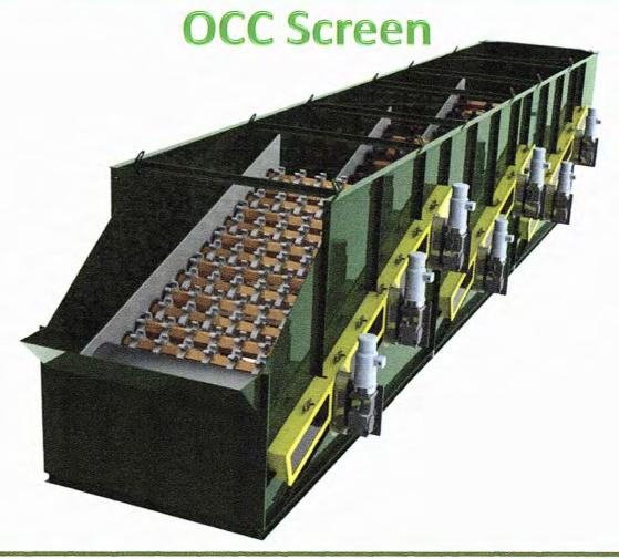
The Green Screens® OCC Screen is designed to separate flat bulky cardboard from competing fiber and 3D containers. Two or three screening decks are offered including two speed zones per deck with variable disc spacing designed to segregate material by size. The OCC discharge conveyor typically includes QC sort locations where sorters can remove contaminates.
