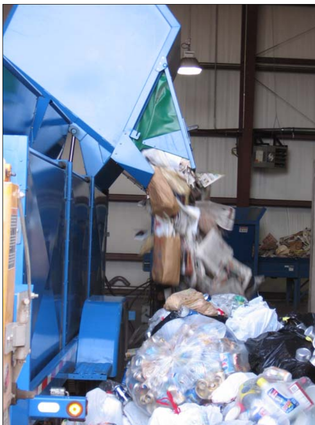
Figure 6 Haul-All Tipping Procedure
