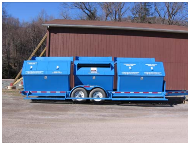
Figure 5 Haul-All Recycling Trailer
