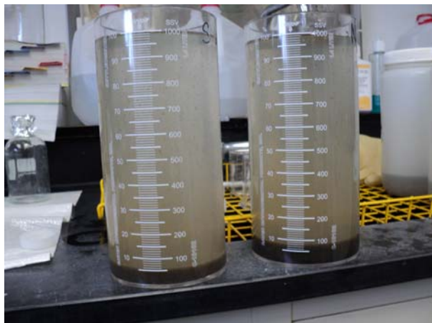
Figure D.1: ½ Hour settleability test results on February 11, 2011
