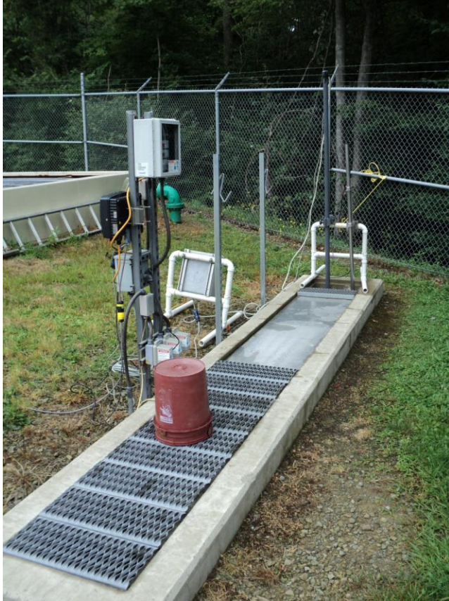
Figure C.3 Locations of Ammonia and Nitrate probes prior to the UV light in the effluent discharge
