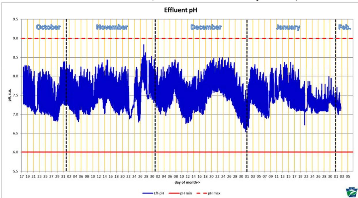
Effluent pH: The probe detected daily pH swings occurring during periods of very low or no flow
