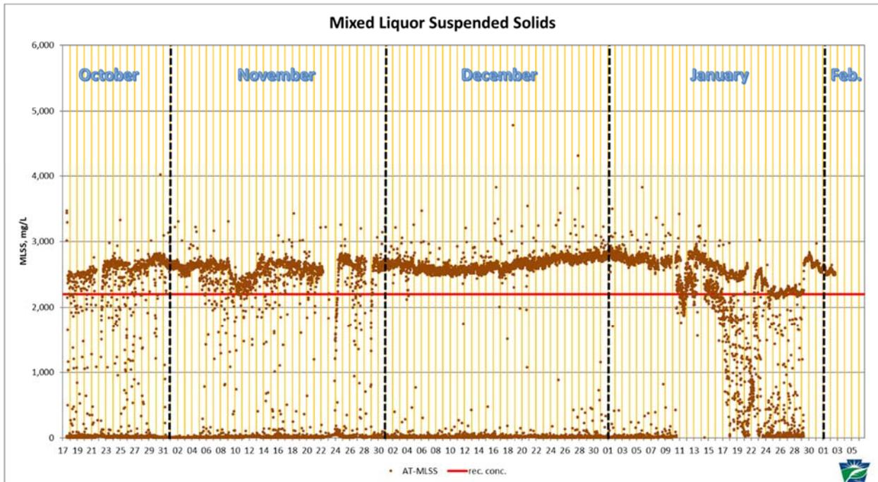
The mixed liquor suspended solids concentration shown here displays solids concentrations generally in the upper 2,000 mg/L range. When aeration was curtailed by the automatic valves, the solids settled into a sludge blanket, dropping below the detection level of the solids probe (thus appearing as zero.) Only during anoxic mixing in January did the solids remain evenly distributed throughout the water column.
