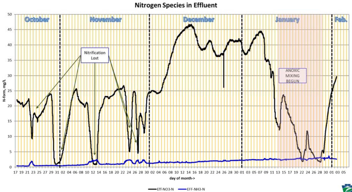
In this chart, the nitrate and ammonium concentrations reflect nitrification losses in October and November, where ammonium increases, nitrites are not formed by the bacteria. Nitrates peaked in December when nitrification succeeded in the presence of magnesia, and this nitrate is seen to be converted to nitrogen gas in January, once the anoxic mixing pumps were installed.
