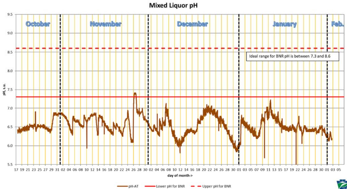
The water of LTMA’s collection system is alkaline deficient, and biological nitrification produces nitrous acid as a byproduct, lowering mixed liquor pH. This pH recording shows that pH was often barely
