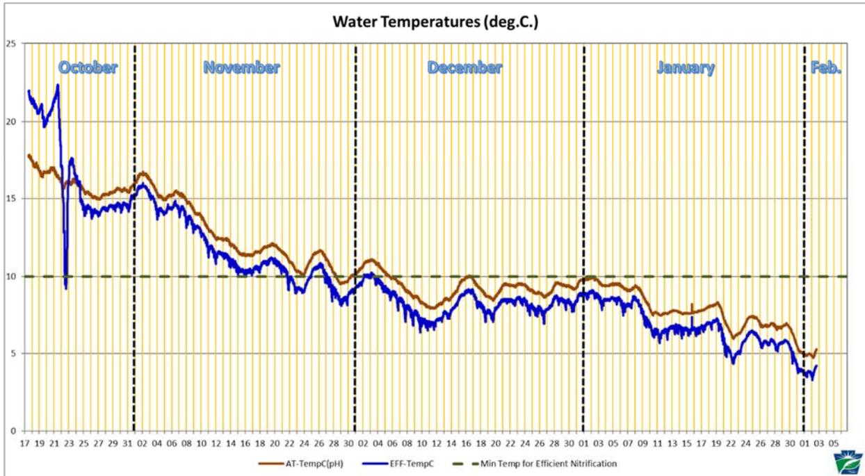
The temperature profile shows decreasing water temperature as winter advances. Since the biomass is temperature-sensitive, its metabolic rate and treatment efficiency falls as the water becomes colder. At 10 deg. C., which is 50 deg. F, nitrification efficiency drops off, and it vanishes below 5 deg. C.
