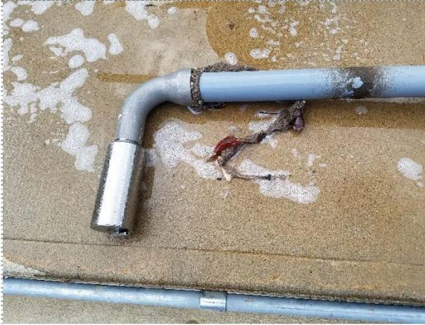
Rag string clinging to solids probe is an example of why fine screening of trash and detritus is necessary for preliminary treatment: rag accumulation on the probe can damage the probe by making the mount too heavy to withstand current forces within the aeration tank.
