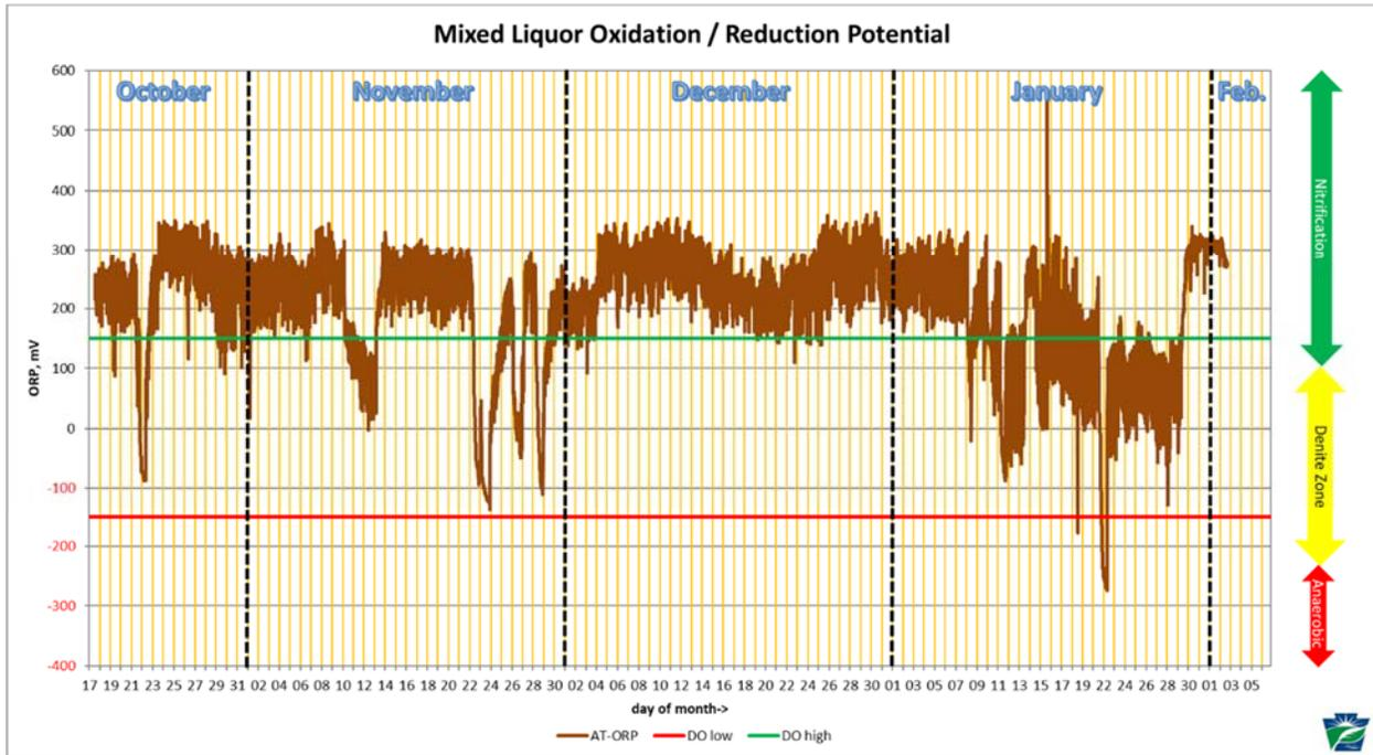
ORP tended to reside in the oxic zone during much of the evaluation. (Oct-early Jan) Once anoxic mixing had begun, the meeting of denitrifier bacteria with both food (BOD) and Nitrate ion under anoxic conditions allowed the bacteria to successfully strip oxygen from the nitrate, reducing nitrogen to molecular nitrogen gas.
