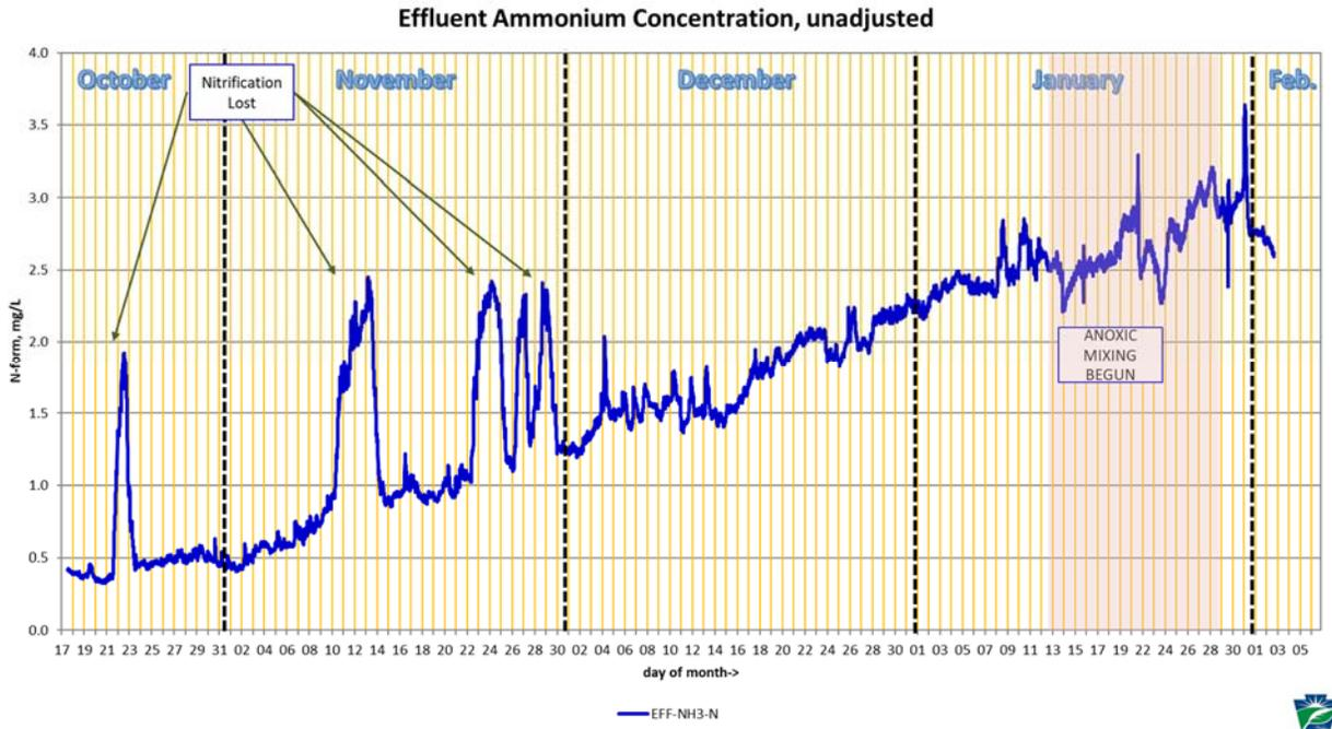
The spikes during October and November represent periods where nitrification was lost due to low influent BOD loading and low aeration alkalinity and pH as noted in the report. Although the ammonium probe became less precise as time passed, it did reflect qualitative improvements in nitrification once the magnesia began to stabilize the biomass under aeration. The gradual rise in ammonium concentration as the winter deepens is a function of decreasing water temperature.
