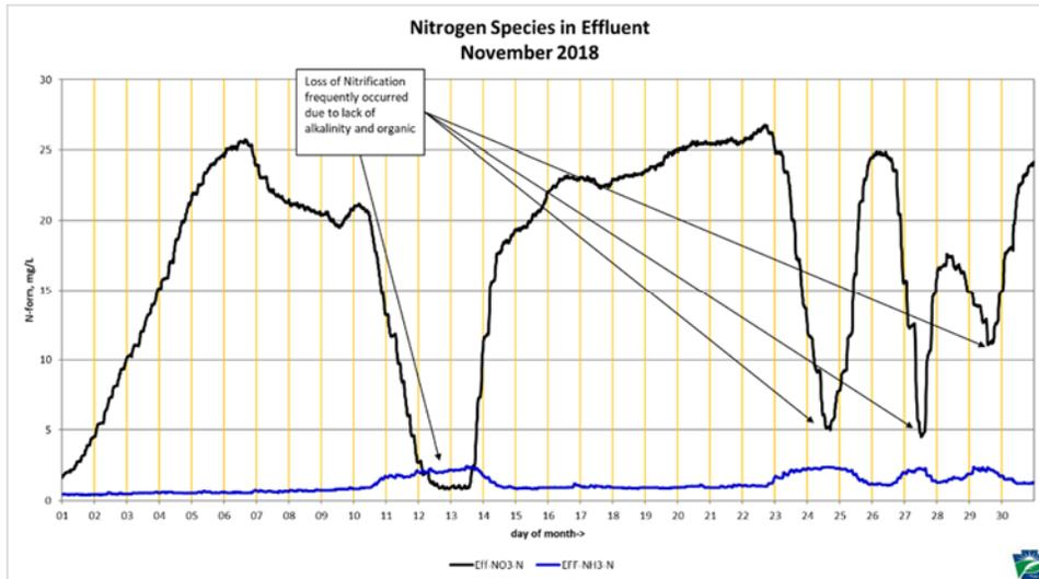
**Graph 2:** November ammonium and nitrate in plant effluent: This shows five (5) incidents of nitrification loss that resulted from decanting of stagnant digester supernate into the aeration tank, which depleted dissolved oxygen while simultaneously overloading the
