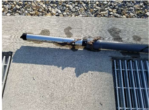
Rags collect on YSI dissolved O2 probe
