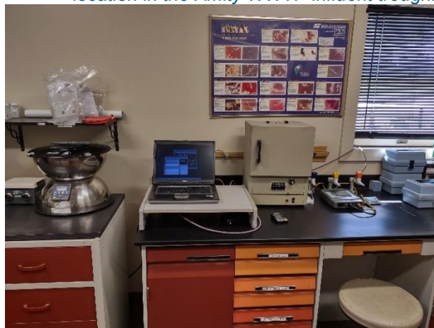
Figure B-9: Photo of PADEP WWTAP process control and bench testing equipment at AMITY WWTF laboratory. The WWTAP laptop includes the data logging and telemetry setup for remote access of data.
