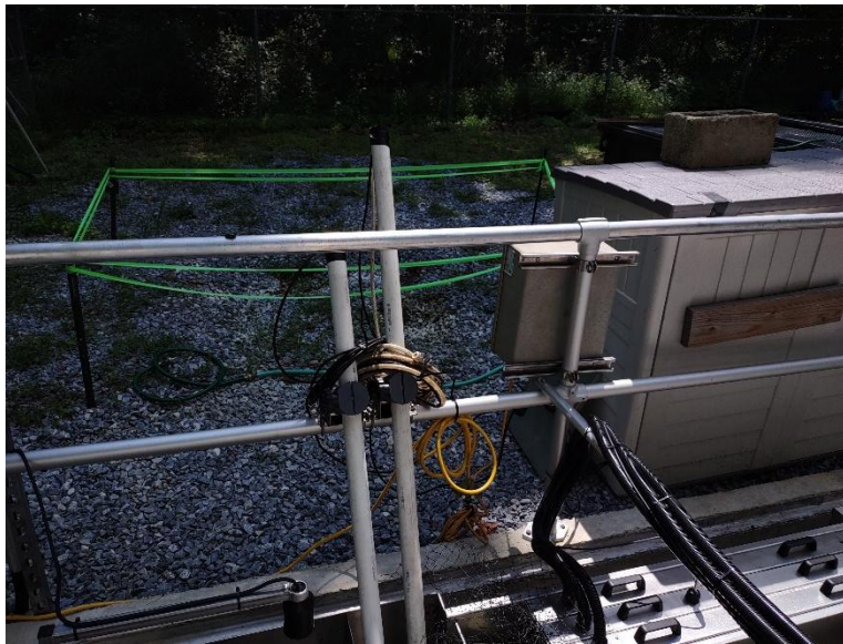
Figure 13) WWTAP continuous monitoring probe placement (Hach AISE and Nitratax) at WWTF final effluent at UV disinfection discharge.
