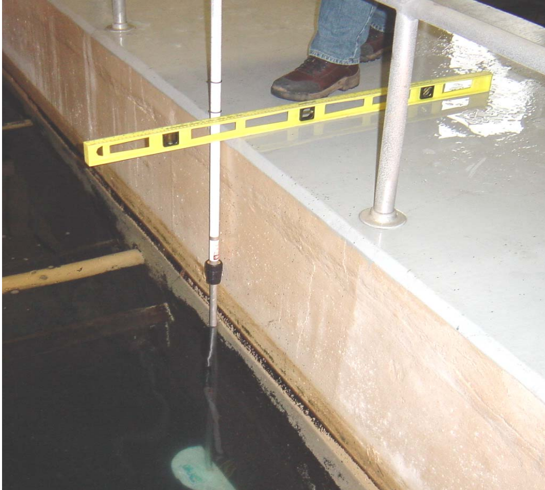
Figure 2. Using a straight edge and a fixed location to record bed expansion measurements. This photo also illustrates the use of the o-rings to record each measurement.
