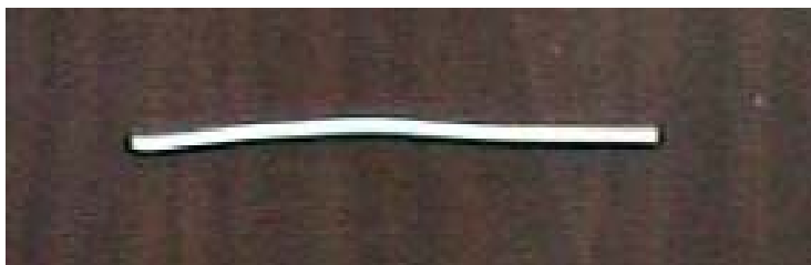
Figure 2.1 Individual Membrane Fiber
