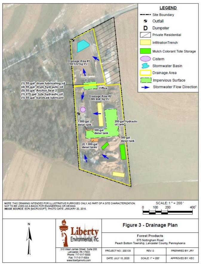
Figure 3. Drainage Plan
