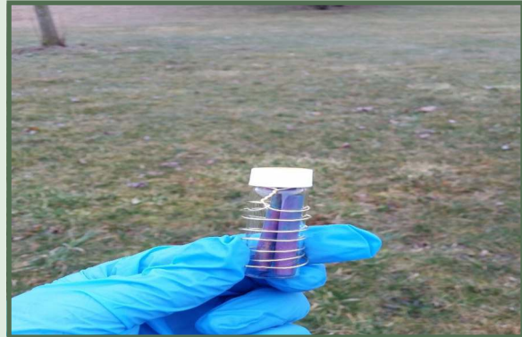
A passive soil gas sampler, prior to being placed in the ground in the area of highest contamination.
