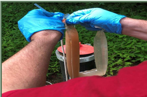
Monitoring wells were sampled with no-purge, passive, disposable plastic sleeve samplers to reduce costs.
