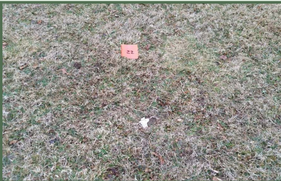
The passive soil gas samplers were covered in aluminum foil, marked with a flag, and then retrieved for analysis after 19 days. No TCE was detected at any of the sampling locations.
