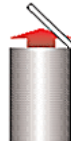
Weak Roof-to-Shell Tank
