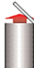
Weak Roof-to-Shell Tank
