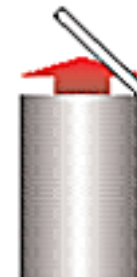
Weak Roof-to-Shell Tank
