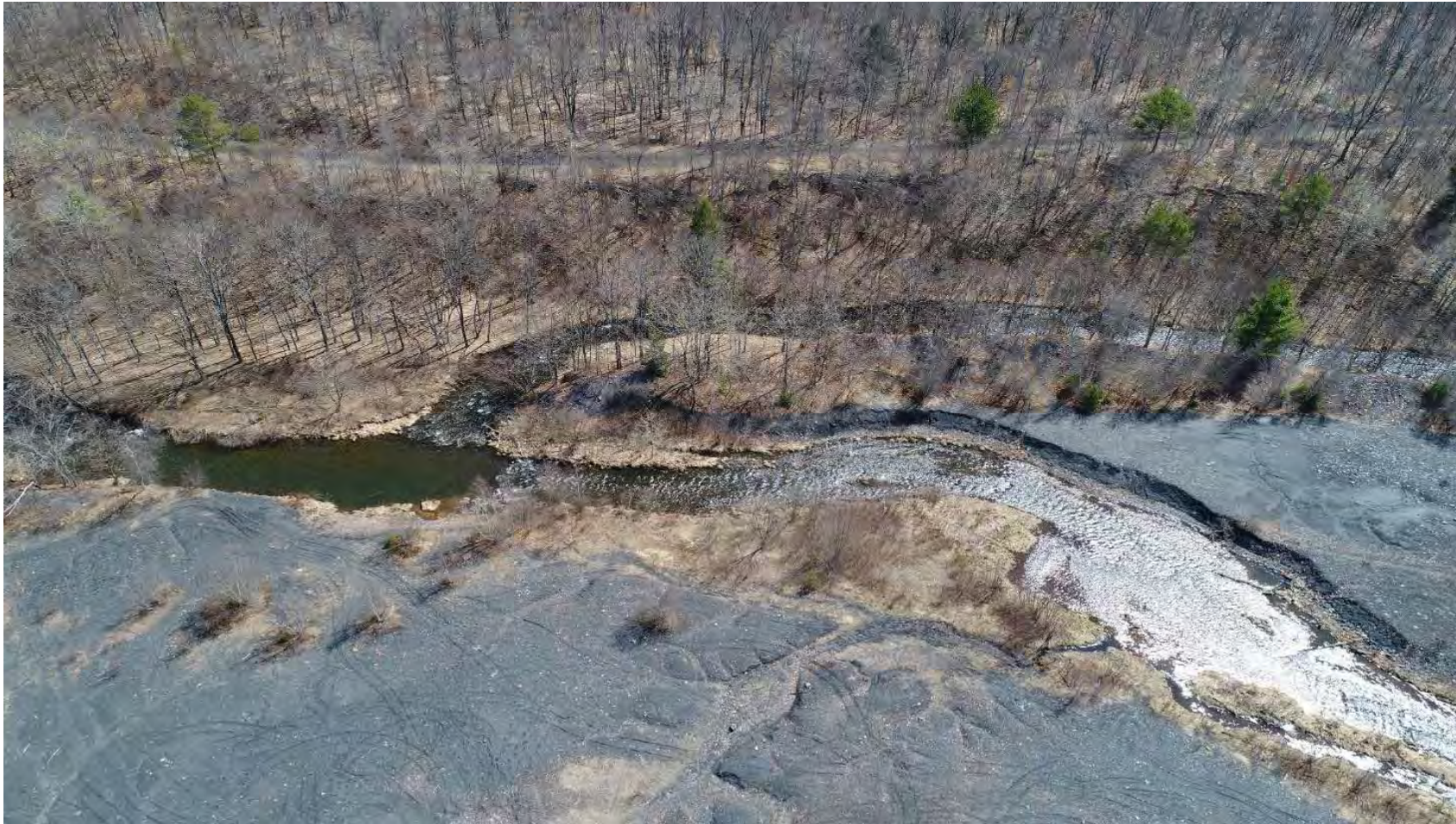
Eroded Stream Channel Diversion
