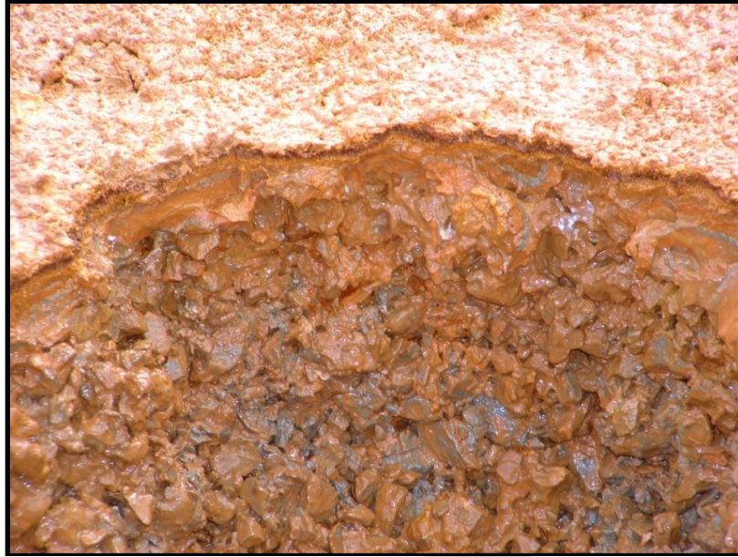
Figure 7.11. Limestone layer clogged with aluminum hydroxide precipitate underneath a relatively clean compost layer in a VFP
