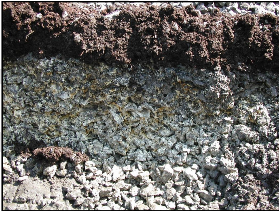
Figure 7.11. Limestone layer clogged with aluminum hydroxide precipitate underneath a relatively clean compost layer in a VFP
