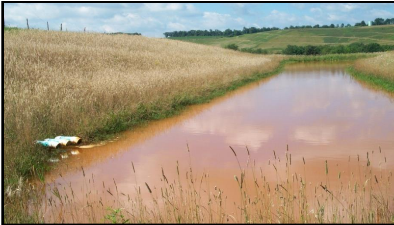
Figure 7.5. Effluent pipes emanating from an ALD followed by an oxidization pond
