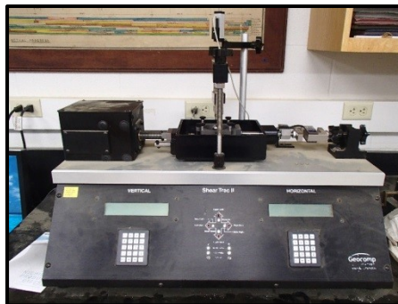
Figure 15 ShearTrac-II Direct Shear Apparatus by Geocomp (from Larson-Robl et al. 2015)
