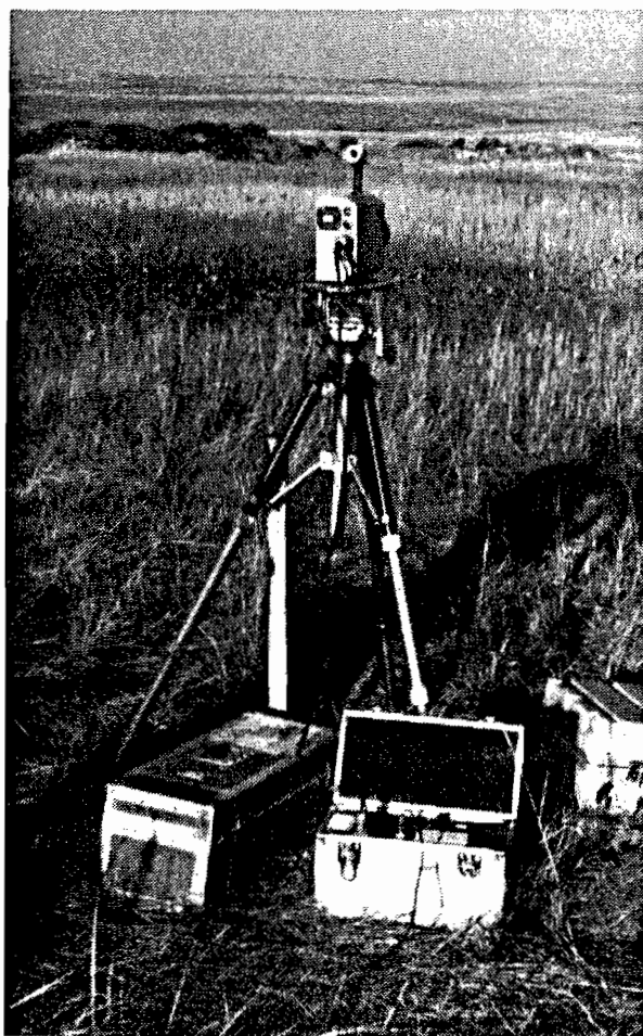
FIG. 6-4: HIGH-SPEED CAMERA SETUP, SHOWING TRIPOD, DC BATTERY PACK AND REMOTE CABLE (LEADING TOWARDS THE PHOTO- GRAPHER)
