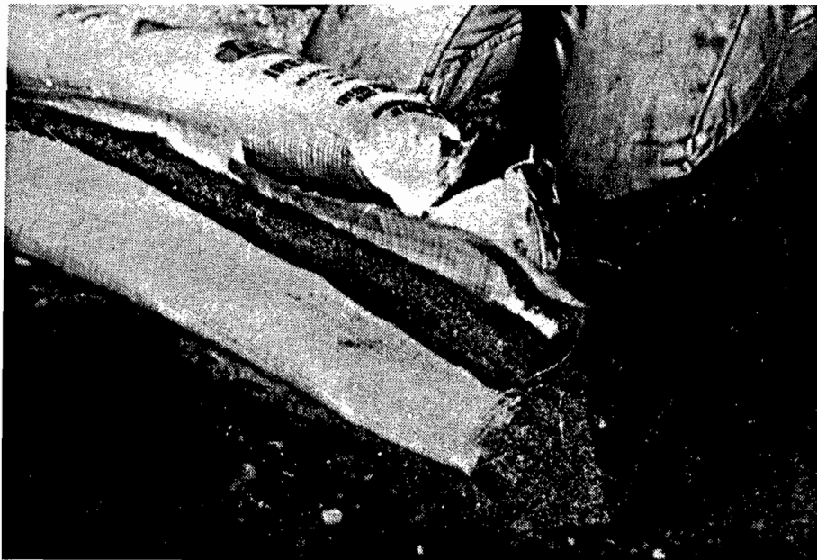
FIG. 5-12: ILLUSTRATING CUT BAG OF IREGEL SLURRY EXPLOSIVE PRODUCT READY FOR LOADING
