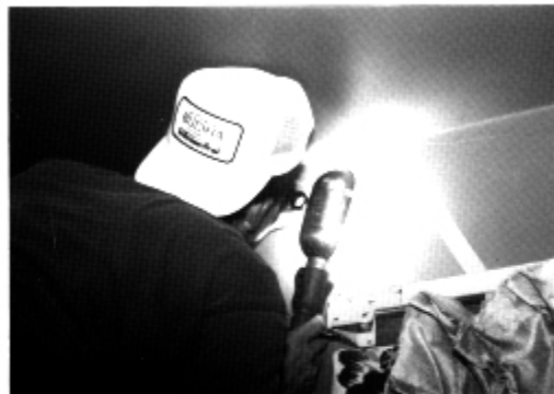
Figure 29. Visual inspections for cracking at the Lhemkuher house showing the optical magnifier and 100 watt sidelight.
