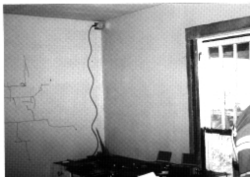
Figure 17. Transducer installed for high corner structural monitoring at the Shack.
