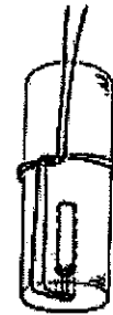
Figure 1: Recommended method of making primer with small diameter cartridge and electric detonator.
