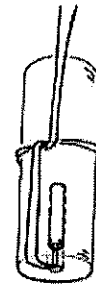
Figure 1: Recommended method of making primer with small diameter cartridge and electric detonator.
