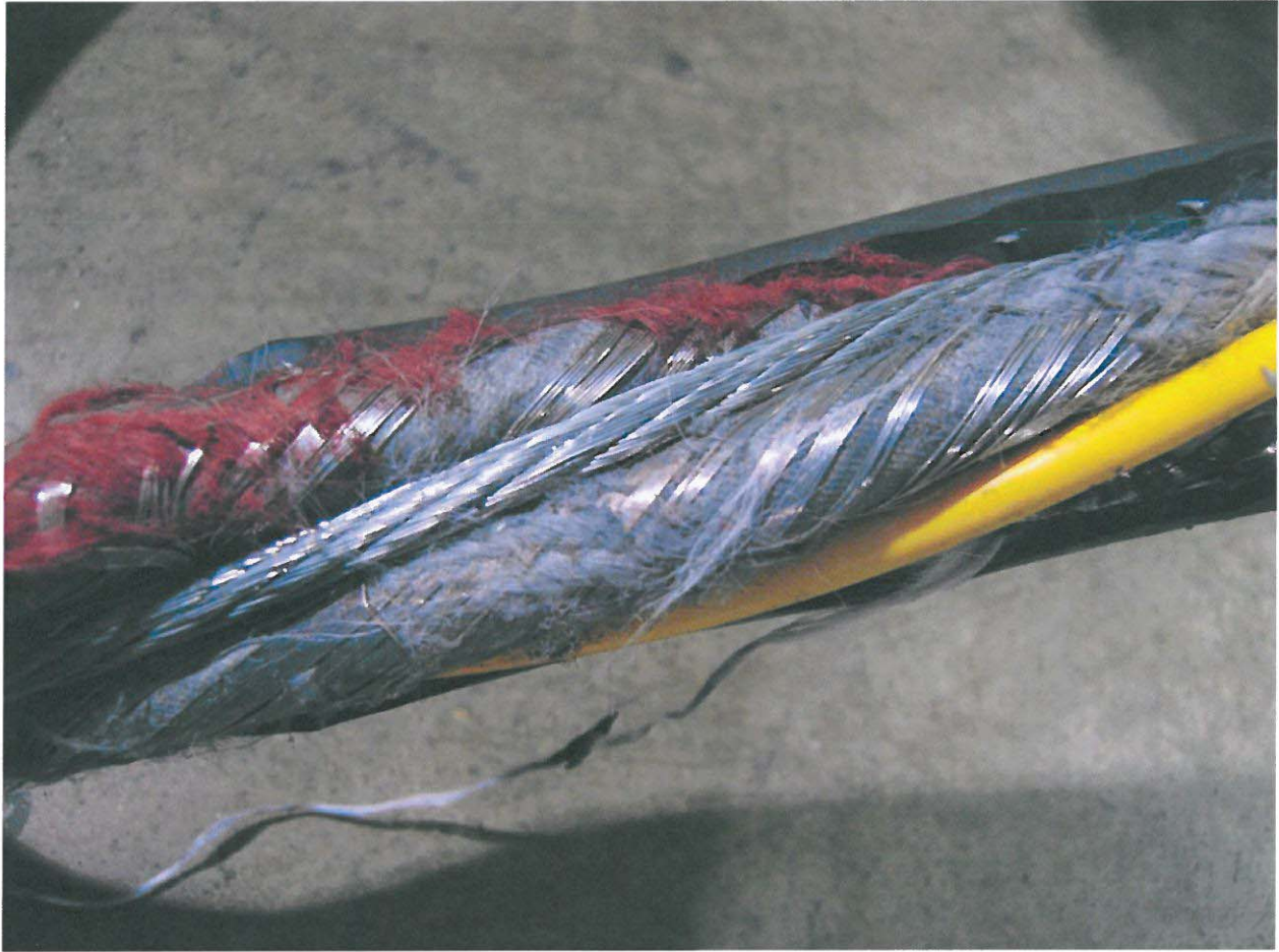
Standard SHDGC with broken shield wires. Also, note the wide spacing of the braid wires after only 3,512 cycles.
