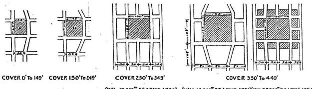
(MIN. 10,000" BEARING AREA) (MIN. 15,600" BEARING AREA)(MIN.ZZ000"BEARING AREA)
