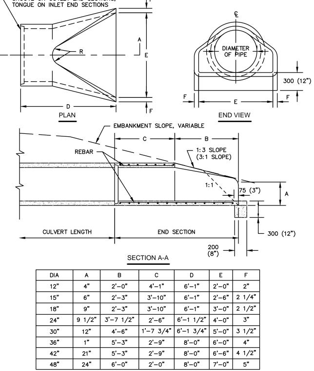
CONCRETE FLARED END SECTION (ROUND PIPE)
