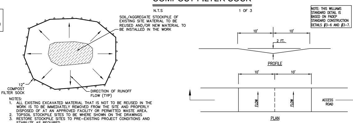
TOPSOIL STOCKPILE SITES TO BE WHERE SHOWN ON THE DRAWINGS 3. RESTORE STOCKPILE SITES TO PRE-EXISTING PROJECT CONDITIONS AND STABILIZE AS REQUIRED. 4. STOCKPILE HEIGHT SHALL NOT EXCEED 35 FEET.
