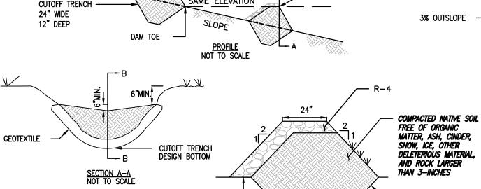
GEOTEXTILE CUTOFF TRENCH INSTALLED ON BOTTOM AND SIDES OF SWALE SECTION B-B NOT TO SCALE
