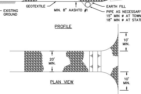
\* MOUNTABLE BERM USED TO PROVIDE PROPER COVER FOR PIPE 1. REMOVE TOPSOIL PRIOR TO INSTALLATION OF ROCK CONSTRUCTION ENTRANCE. EXTEND ROCK OVER FULL WIDTH
