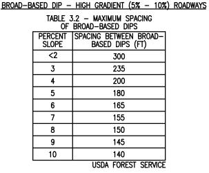
BROAD-BASED DIPS SHALL BE CONSTRUCTED TO THE DIMENSIONS SHOWN AND AT
