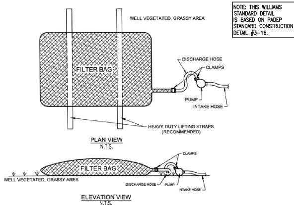
LOW VOLUME FILTER BAGS SHALL BE MADE FROM NON-WOVEN GEOTEXTILE MATERIAL SEWN WITH HIGH STRENGTH, DOUBLE STITCHED "J" TYPE. THEY SHALL BE CAPABLE OF TRAPPING PARTICLES LARGER THAN 150 MICRONS. HIGH VOLUME FILTER BAGS MAY BE MADE FROM WOVEN GEOTEXTILES THAT MEET THE FOLLOWING STANDARDS:
