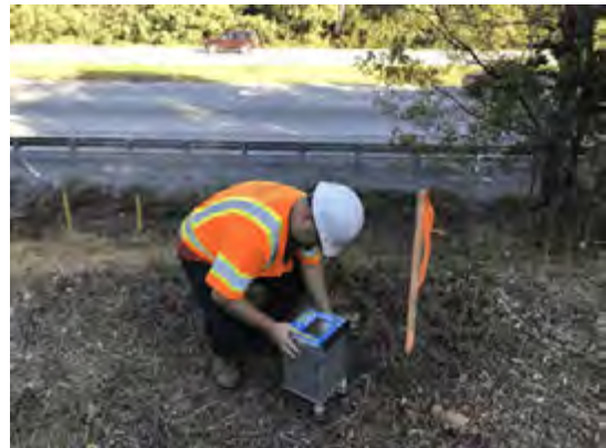
Making a gravity measurement with the CG-5 on the HDD 400 alignment.
