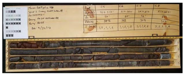
**Photograph 2:** B2-6E, Samples C-5 to C-8 (46.4 to 66.4 feet)
