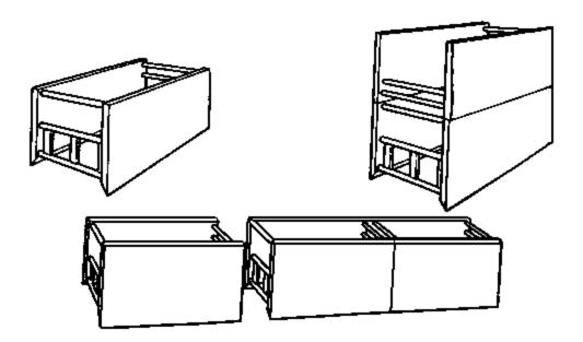
Figure 4. Trench Shields
