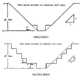
3. All excavations 20 feet or less in depth which have vertically sided lower portions shall be shielded or supported to a height at least 18 inches above the top of the vertical side. All such excavations shall have a maximum allowable slope of 1:1.
