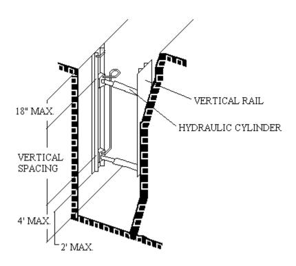
Figure 1. Aluminum Hydraulic Shoring
