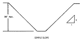
2. All benched excavations 20 feet or less in depth shall have a maximum allowable slope of 1:1 and maximum bench dimensions as follows:
