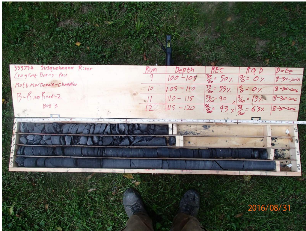
Figure B-RR-2.5 B-RiverRoad-2 Box 3 Runs 9-12 Dry
