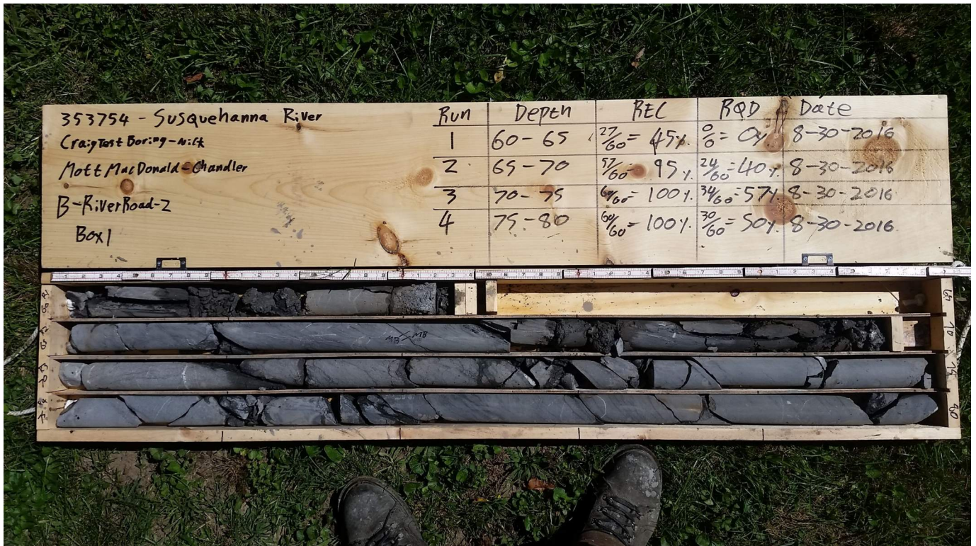
Figure B-RR-2.1 B-RiverRoad-2 Box 1 Runs 1-4 Dry
