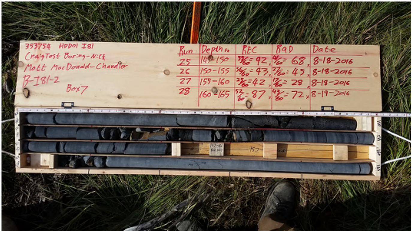
Figure B-I81-2.13 B-I81-2 Box 7 Runs 25-28 Dry
