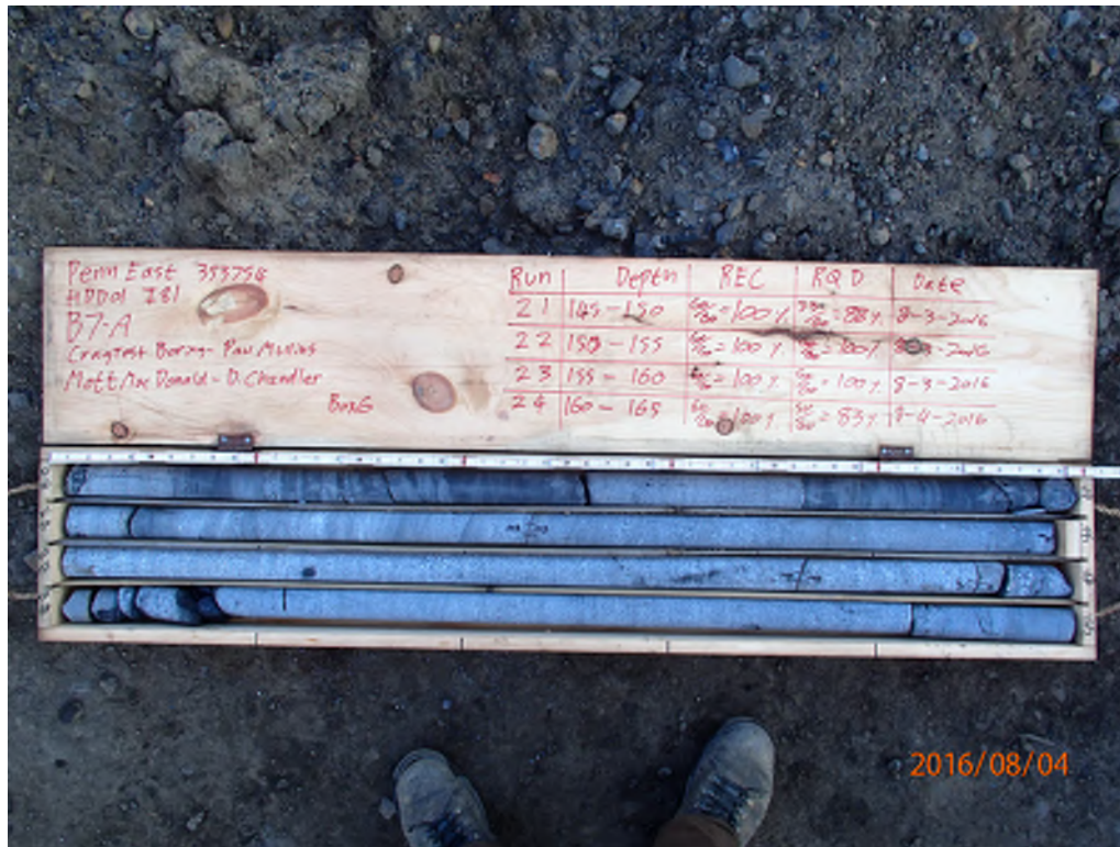
Figure B-7A.11 B-7A Box 6 Runs 21-24 Dry
