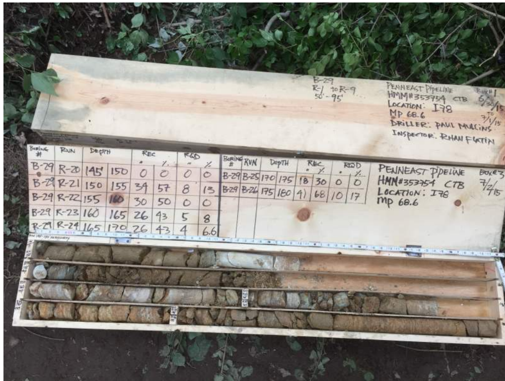
Figure B-29.5 B-29 Box 3 Run 20-26 Dry
