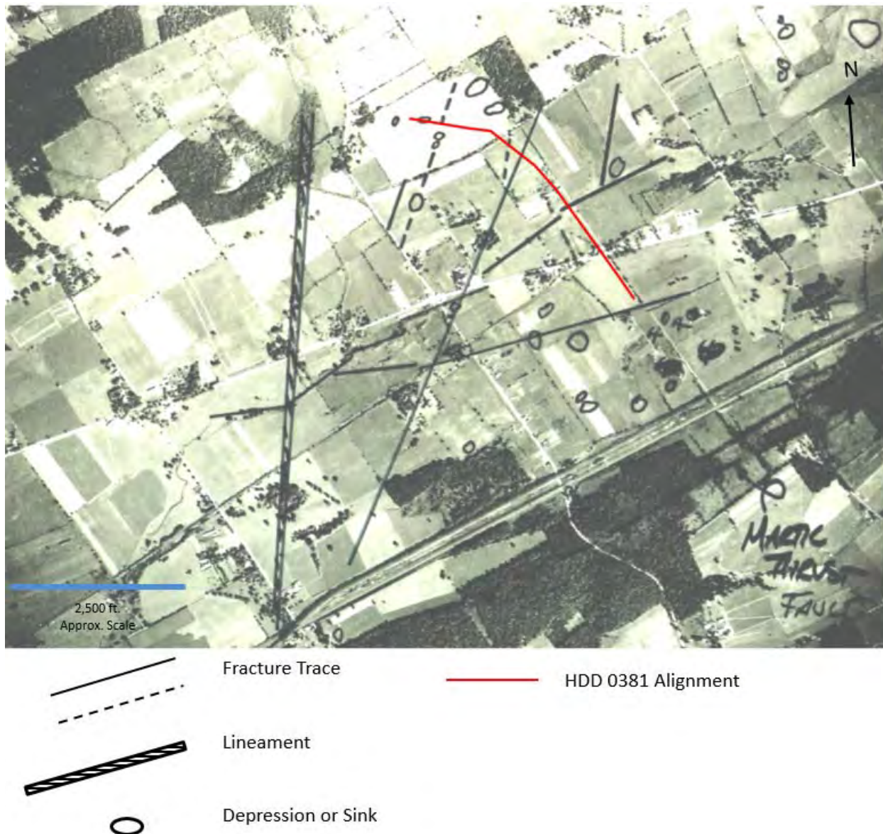
Figure 3. Fracture Trace Mapping in Area of HDD S3-0381
