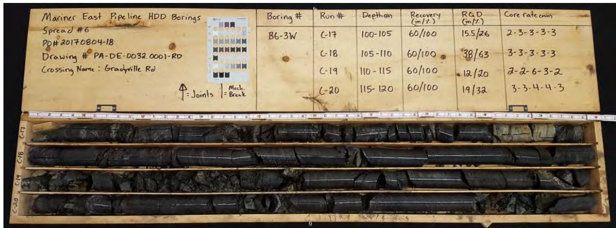
Photograph 5: B6-3W, Samples C-17 to C-20 (100 to 120 feet)
