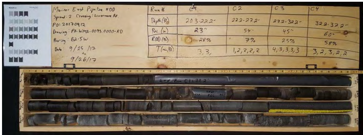
Photograph 1: B2-5W, Samples C-1 to C-4 (20.3 to 37.2 feet)
