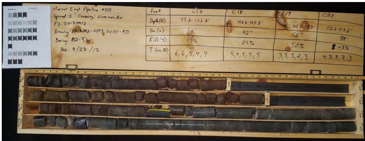
Photograph 5: B2-5W, Samples C-17 to C-20 (97.2 to 117.2 feet)
