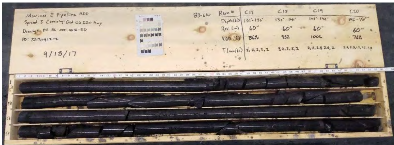
Photograph 5: B3-6W, C-17 to C-20 (131 to 151 feet)
