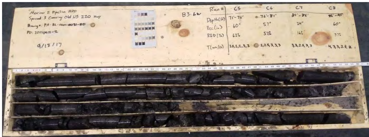
Photograph 2: B3-6W, Samples C-5 to C-8 (71 to 91 feet)
