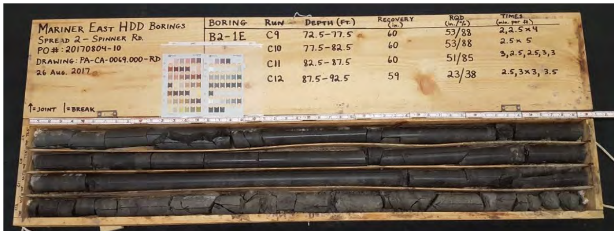
Photograph 3: B2-1E, Samples C-9 to C-12 (72.5 to 92.5 feet)
