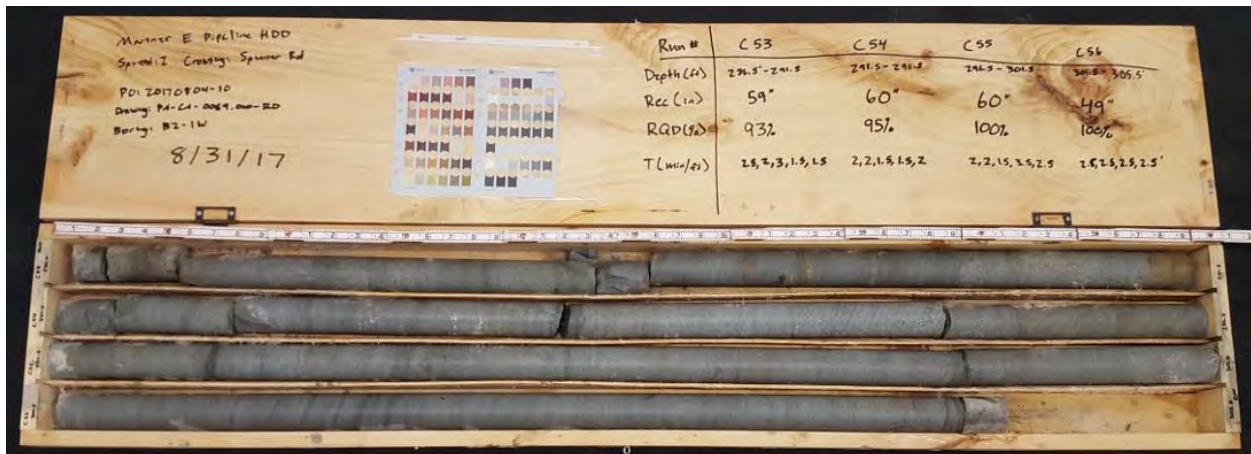
Photograph 14: B2-1W, Samples C-53 to C-56 (286.5 to 301.5 feet)
