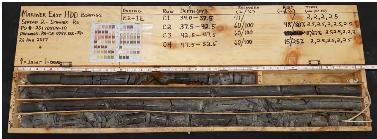
Photograph 1: B2-1E, Samples C-1 to C-4 (34 to 52.5 feet)
