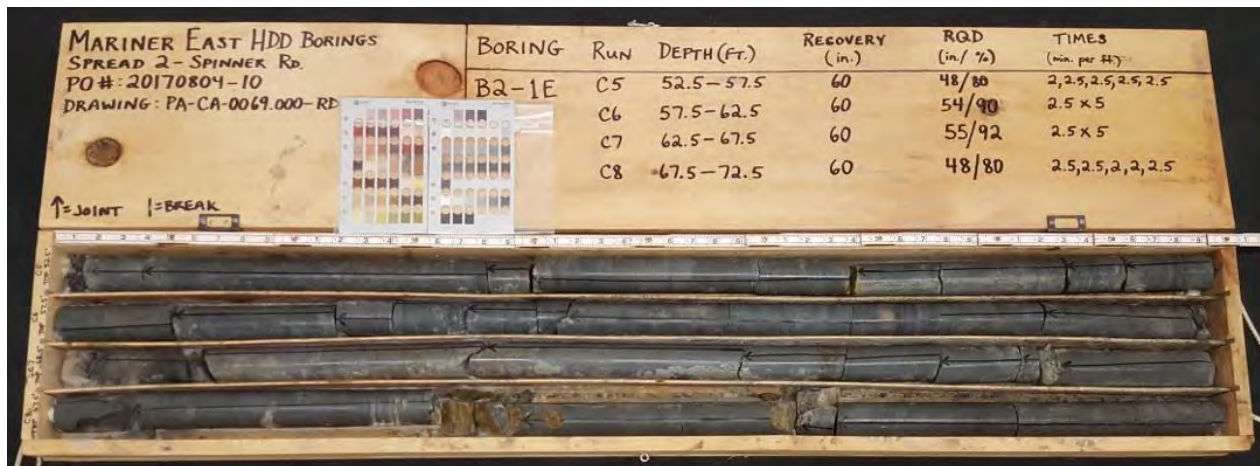
Photograph 2: B2-1E, Samples C-5 to C-8 (52.5 to 72.5 feet)
