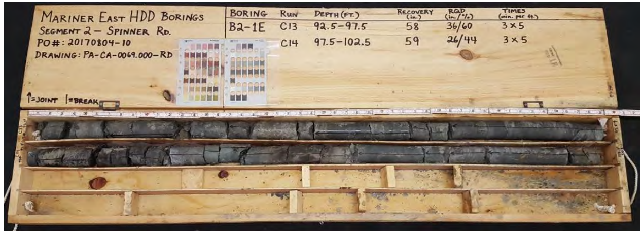
Photograph 4: B2-1E, Samples C-13 to C-14 (92.5 to 102.5 feet)
