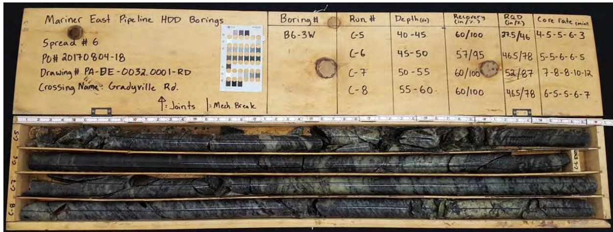
Photograph 2: B6-3W, Samples C-5 to C-8 (40 to 60 feet)
