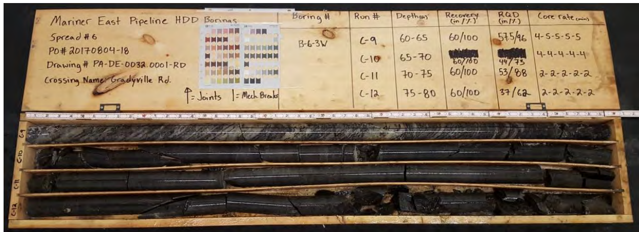
Photograph 3: B6-3W, Samples C-9 to C-12 (60 to 80 feet)
