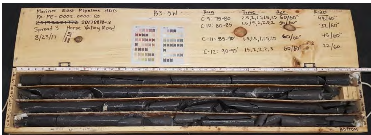
Photograph 3: B3-5W, Samples C-9 to C-12 (75 to 95 feet)
