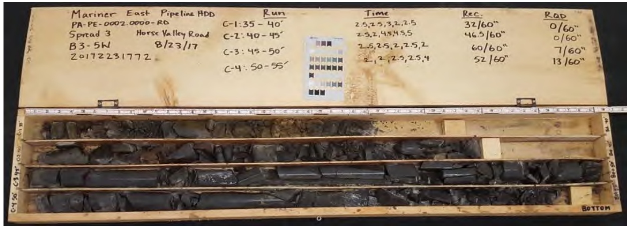
Photograph 1: B3-5W, Samples C-1 to C-4 (35 to 55 feet)
