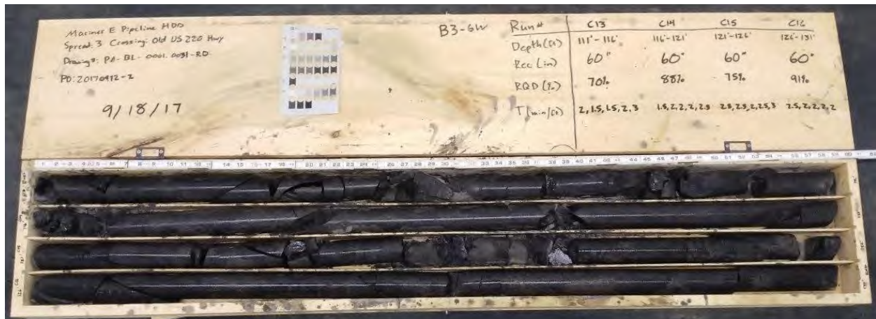
Photograph 4: B3-6W, Samples C-13 to C-16 (111 to 131 feet)
