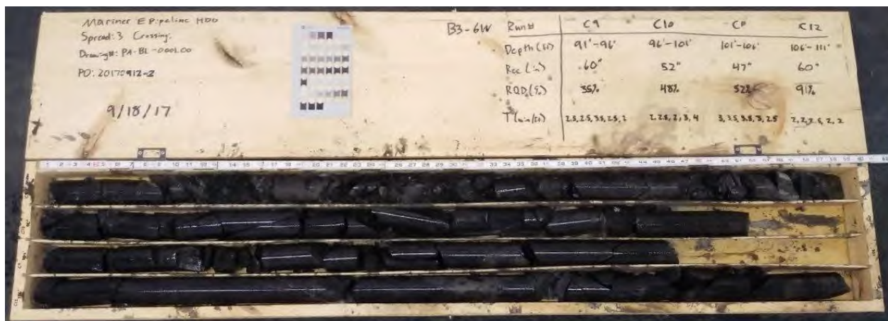
Photograph 3: B3-6W, Samples C-9 to C-12 (91 to 111 feet)
