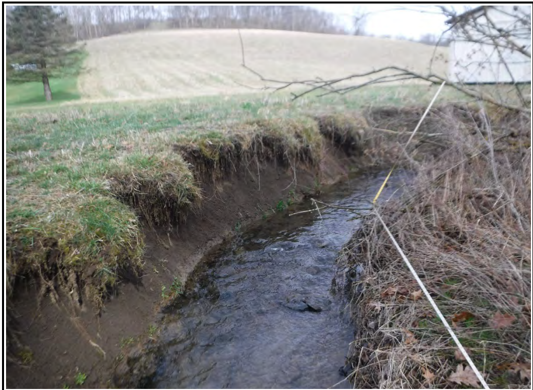
Photograph 2: Eroded right descending bank in lower section of station FR-1 (March 18, 2020)
