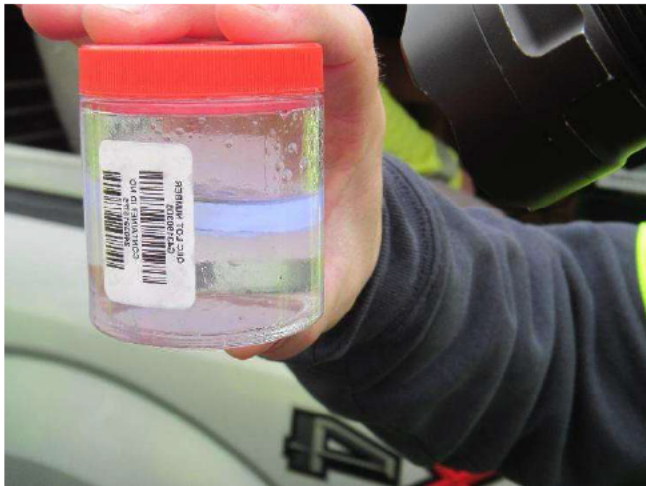
Photo 3: Product sample showing UV staining
