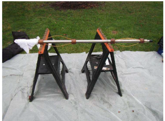
Photo 4: Advanced Logic Technology (ALT) QL40-OB12G-UV Optical Televiwer (OPTV) with ultraviolet (UV) imaging capabilities
