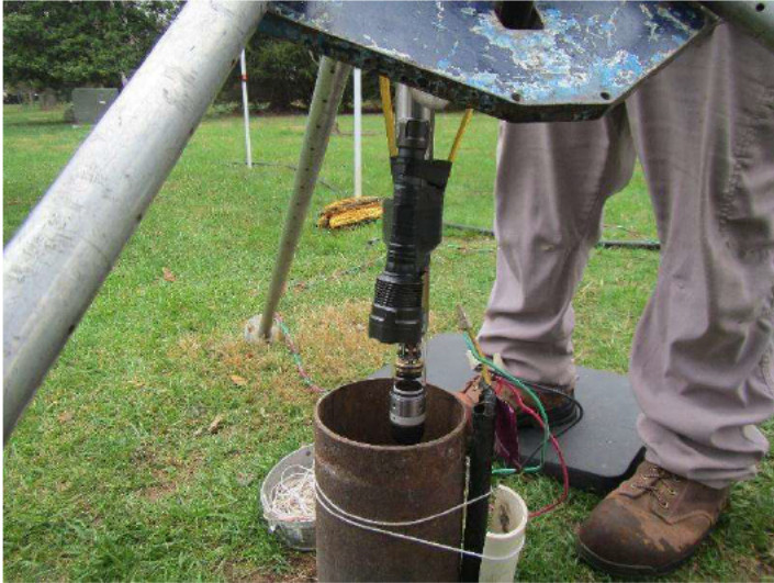
Photo 5: inserting the tool with UV flashlight taped
