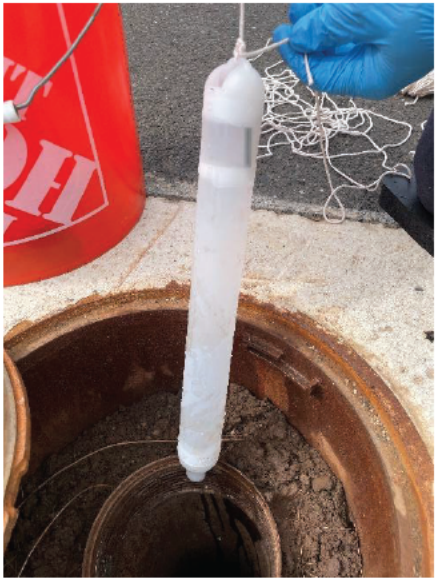
Photo 1: RW-4 Bailer Check Side View
