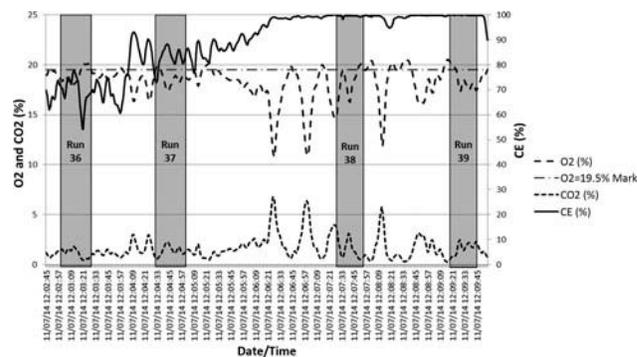
**Figure 3.** Example O<sub>2</sub>, CO<sub>2</sub>, and CE data from extractive method overlaid with imager test time for test numbers 36, 37, 38, and 39.
