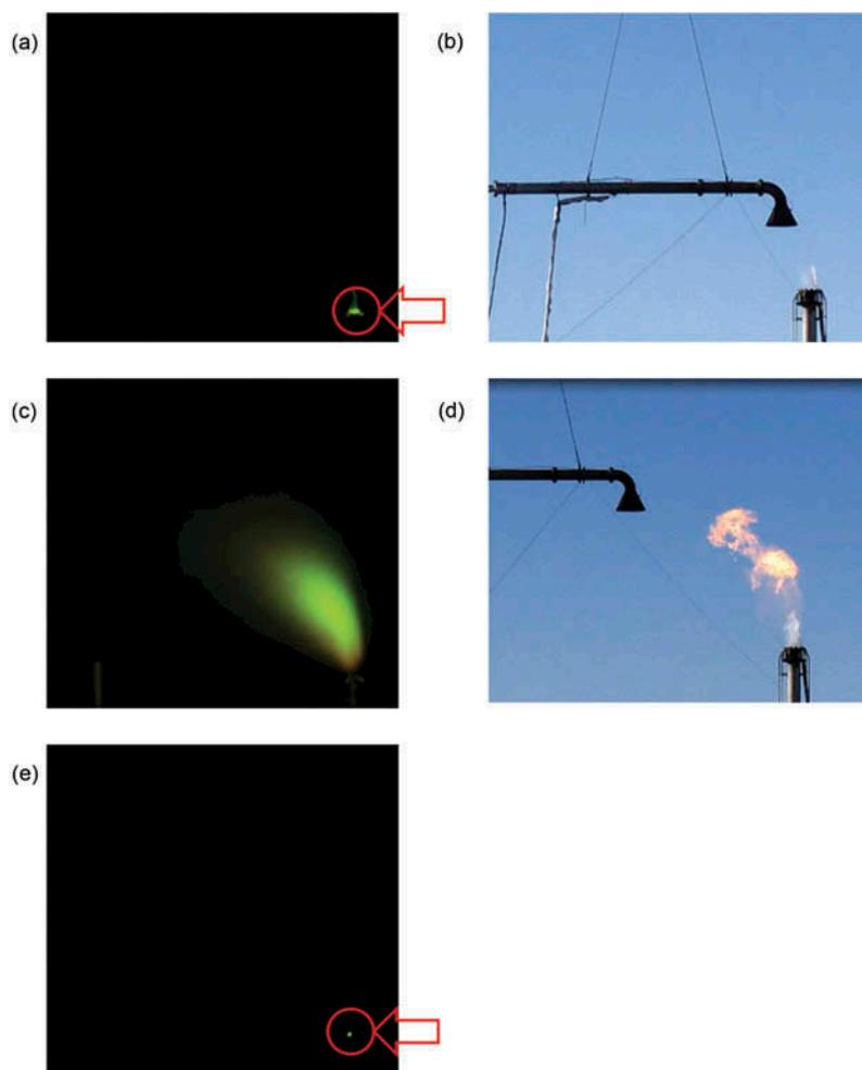
**Figure 6.** Images of small flare sizes and pilot: (a) IR image of Test 19; (b) visible image of test 19; (c) IR image of test 18; (d) visible image of test 18; and (e) IR image of test 13—no vent gas, lit pilot only.
