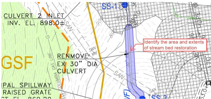
10. §102.4(b)(5)(ix), §102.8(f)(9): The floodway limits on all streams are depicted with widths less than 50-feet and in some cases appears to differ from what has been provided with the USACE/PADEP Joint (Joint) permit application. Please update the floodway limits shown as well as all other information provided within the plan drawings to reflect changes made during the Joint permit application review(s).
